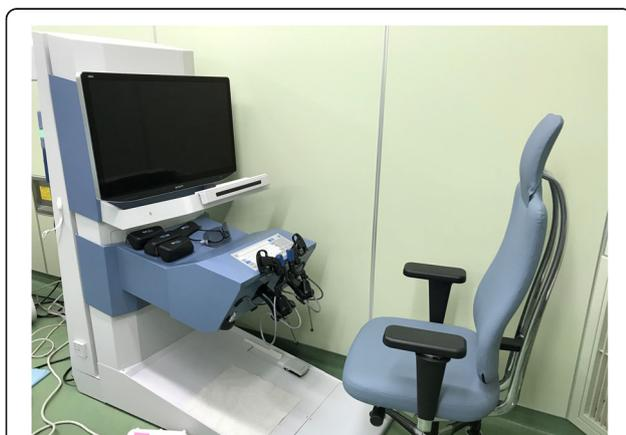
**Fig. 4** A system of the remote control unit called a cockpit
